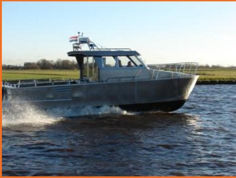
The OrangePit StrongCat 10.0 is a fast, all weather aluminum workboat which is sturdy build and can be equipped with stern drive or water jet propelled by Yanmar inboard diesel engines
